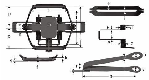
In order to reduce the risk of measurement errors and to ensure consistency, it is recommended that each trap component measurement be taken four times on each trap.
